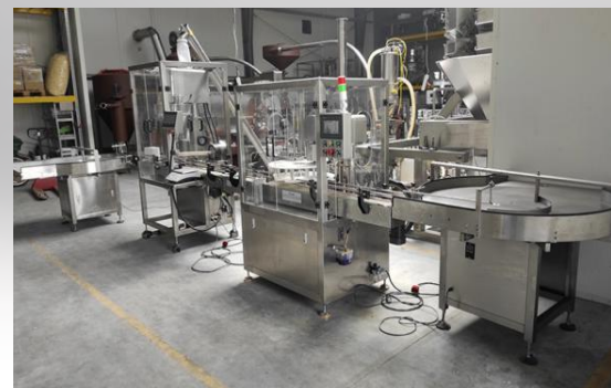
Powder dosing station SDP/S 500 A + Flat rotary table conveying/receiving 1200S/S
