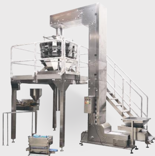
Packing line: DWK/W/S 14 M + PWK 2000/2000 + PRZ 3750 + thick liquid filler DPG/S 1000
