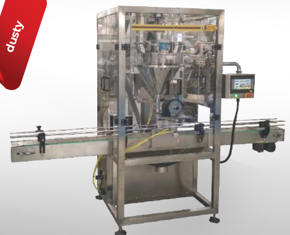
Packaging line for powdery products into tubes SDP/S 500 A
