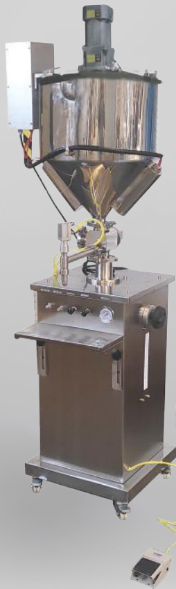
Free-standing thick liquid filler DWPG/S HOT (heating device HOT)
