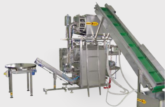
Packing line: Filler with sauerkraut feeder DKK 1000 + COFPACK P/S 60/500 + OGT/S 300 + rotary table
