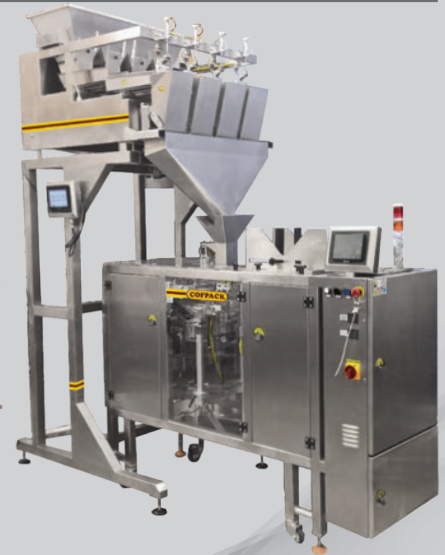
Packing line: COFPACK MULTI 160/300 U + DWL 4 + stand
