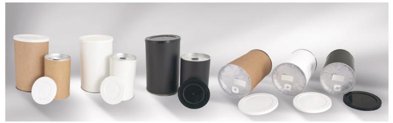
Standard cardboard TUBES. Also available as an option with a valve. The packages are made of cardboard glued with a thickness of  $\sim$  1.1 mm. The interior is lined with aluminum foil. The tubes are equipped with an aluminum membrane with a handle for easy opening. Sold complete with a plastic lid and a metal bottom for self-assembly.
